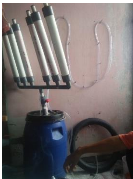
Gambar 1. Alat Biogas Purifier
