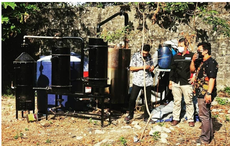
Gambar 3 Persiapan Peralatan Pirolisis 500 L 2 Fire Channel
